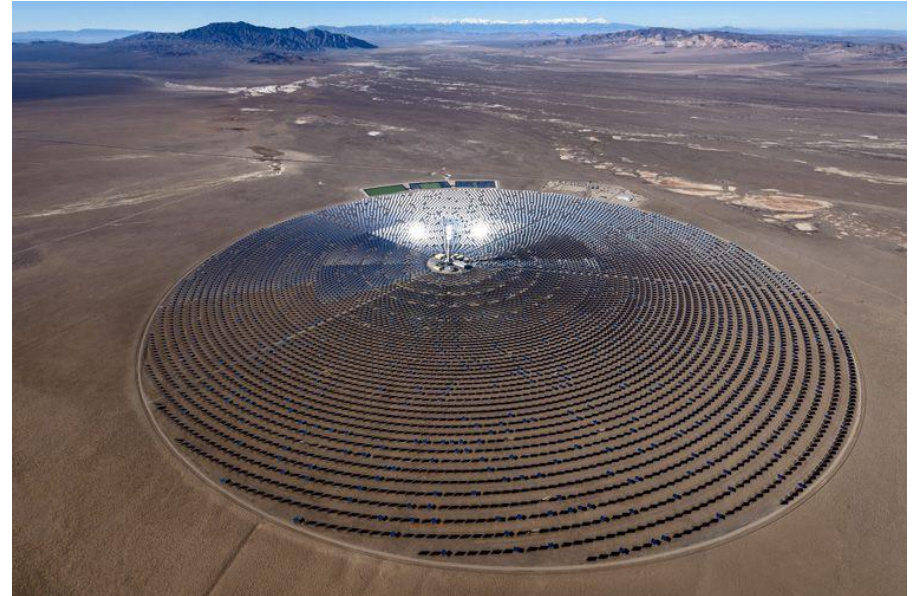
Tower using molten salts CRESCENT DUNES (Solar Reserve) February 2016 110 MWe, 10 h thermal storage (Nevada, USA)
